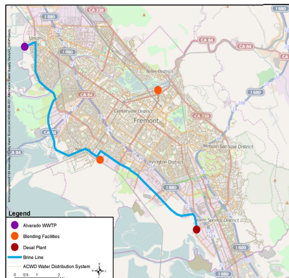
Figure 5-6 Bay Desalination Concept with Brine Discharge Line
