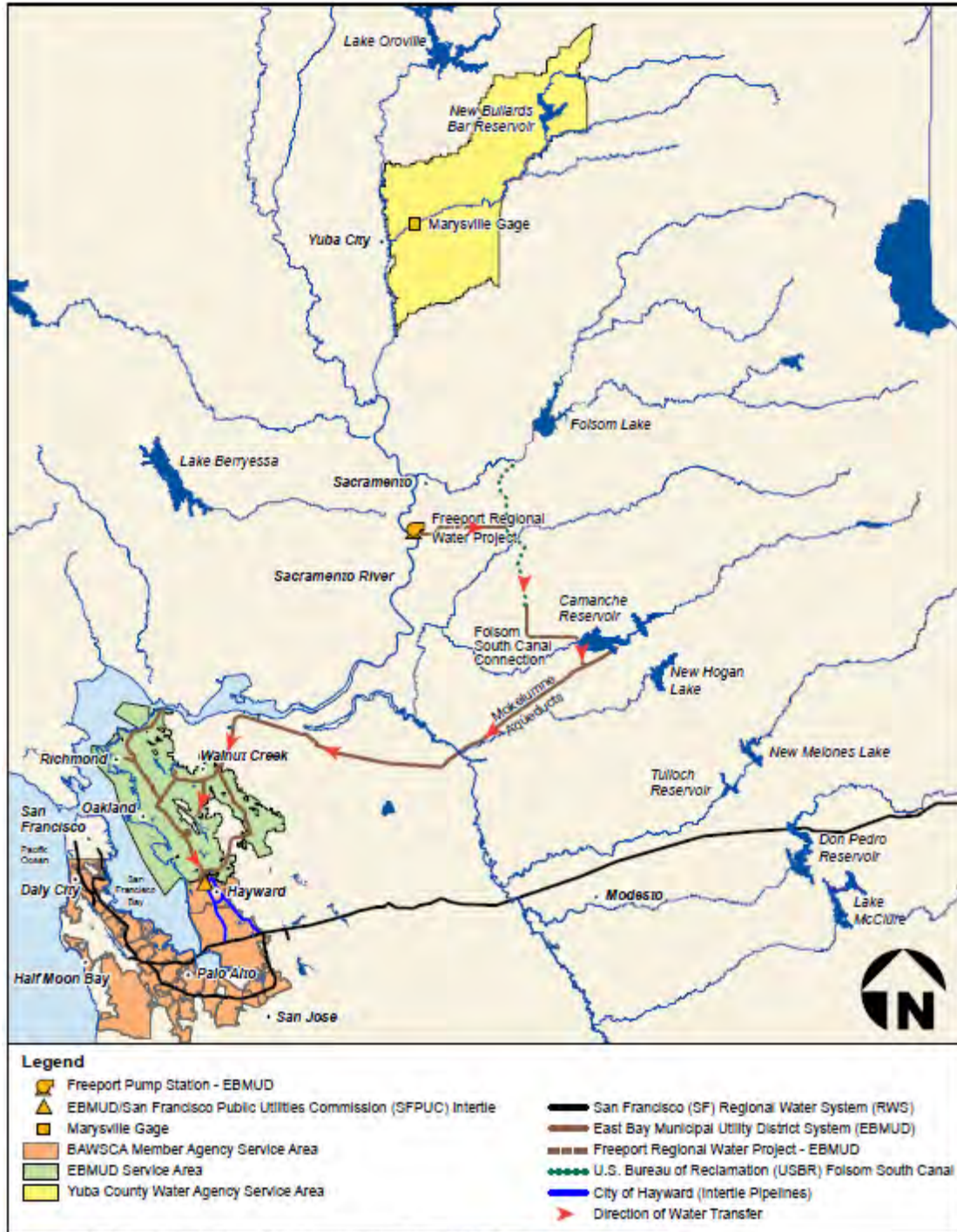
Figure 1. Map Showing the Existing Infrastructure that to Support a Pilot Water Transfer and the Direction of the Water Movement through EBMUD’s System.
