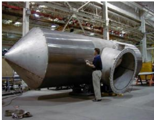
Figure B-4 Passive Screen Illustration and a Picture of a Large-Diameter Passive Wedgewire Screen (Courtesy of Johnson Screens)
