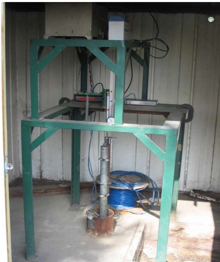
Figure 7-4. San Jose (“Martha”) Extensometer
