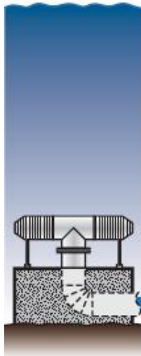
Figure B-4 Passive Screen Illustration and a Picture of a Large-Diameter Passive Wedgewire Screen (Courtesy of Johnson Screens)
