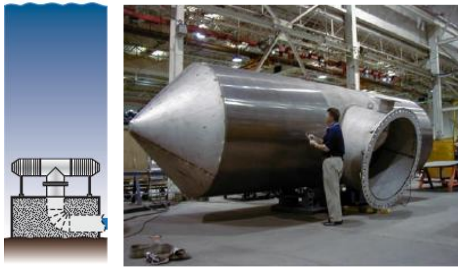
Figure C-6 Passive Screen Illustration and a Picture of a Large-Diameter Passive Wedgewire Screen (Courtesy of Johnson Screens)
