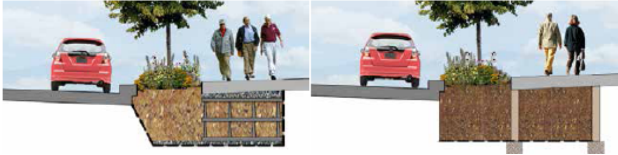
Figure 2-2 Stormwater tree well filter conceptual examples: modular suspended pavement system (left), column suspended pavement system (right). (Courtesy of City of Philadelphia Water Department)
