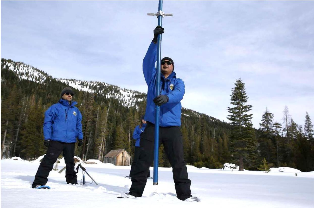
*Sean DeGuzman of the state Department of Water Resources uses a metal tube to calculate the depth and water content of the Sierra snowpack at Phillips Station near Lake Tahoe.*
