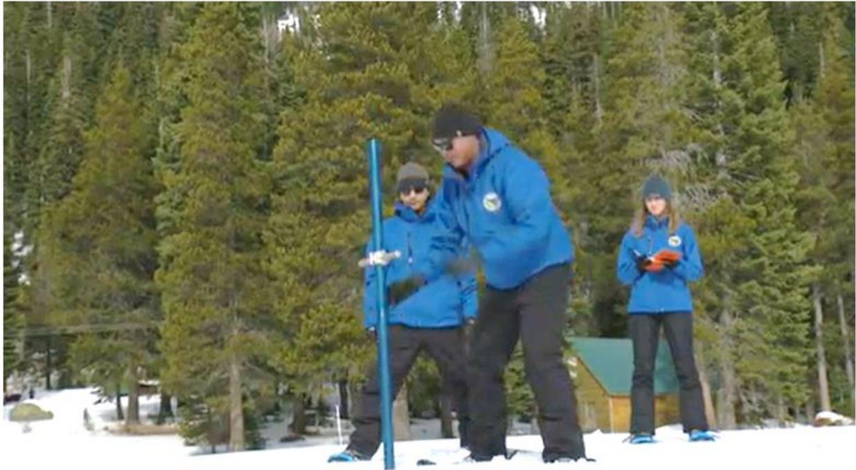
*The CA Department of Water Resources conducted the first manual snow survey of 2020 on Jan. 2, 2019. They recorded 33.5 inches of snow depth and a snow water equivalent of 11 inches, which is 97 percent of average for this location. BY CALIFORNIA DEPARTMENT OF WATER RESOURCES*
